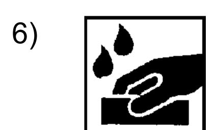
Schleifen (naß) Rub down (wet) Poncer (mouillé)
